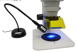
The light head, barrier filter, and filter shield are interchangeable so that you can easily switch between excitation/emission light+filter combinations.
